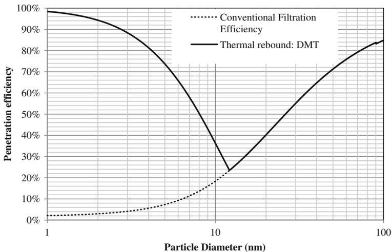
Fig. 13.7 Calculated penetration efficiency using DMT model
