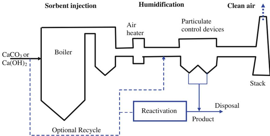
**Fig. 9.4** A typical furnace sorbent injection process
