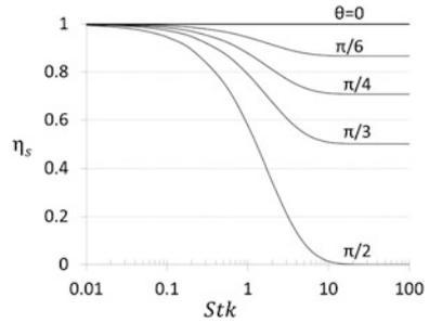
**Fig. 15.8** Misalignment sampling efficiency when  $R \neq 1$  ( $\theta = \pi/3$ )
