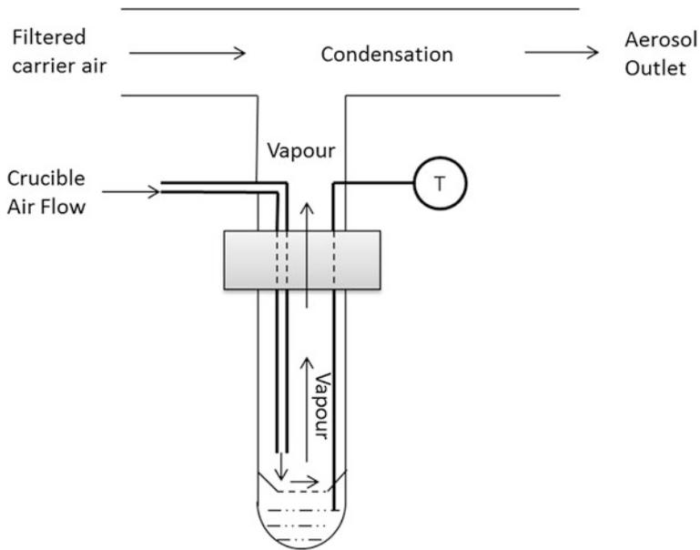
**Fig. 13.9** Evaporation–condensation technique for nanoaerosol generation [15]
