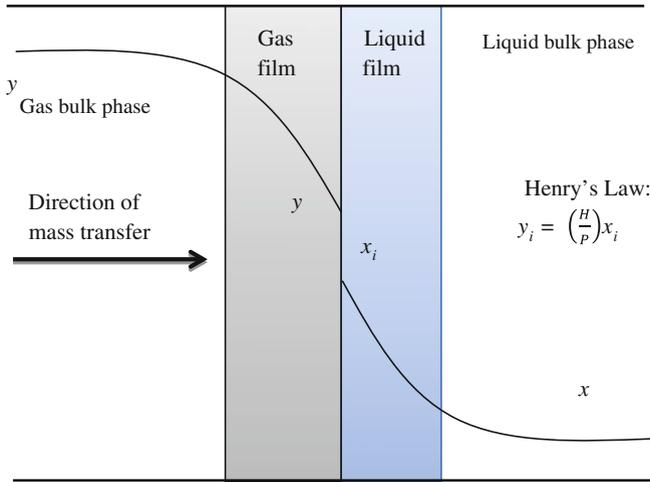
**Fig. 2.9** Gas–liquid interfacial mass transfer two-film theory
