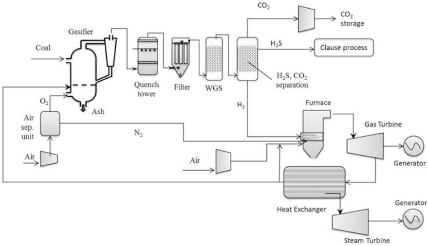
**Fig. 12.1** Simplified IGCC with pre-combustion CO<sub>2</sub> capture process
