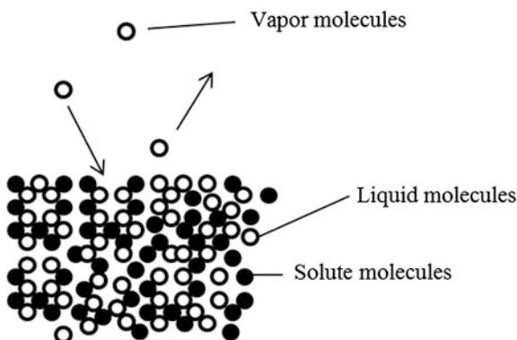
**Fig. 2.8** Vapor pressure of a nonideal solution
