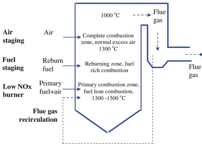
Fig. 9.11 Principles of low-NO<sub>x</sub> formation approaches
