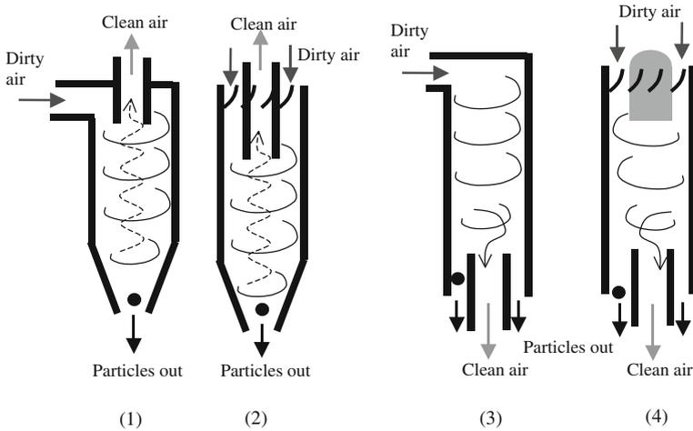
**Fig. 6.7** Schematics of four types of cyclones (Source [42])
