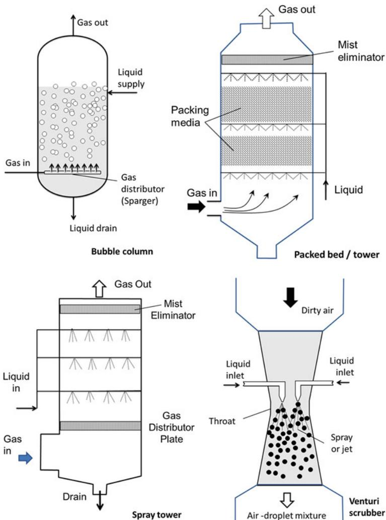
Fig. 10.5 Schematic diagram of typical wet scrubbers
