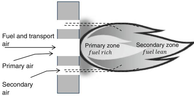
**Fig. 9.8** Air staging in a burner
