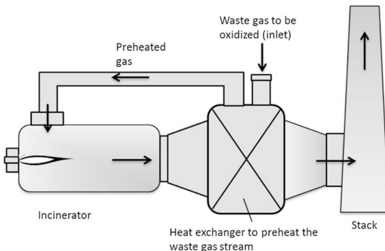
**Fig. 10.7** A typical thermal VOC incinerator with recuperative heat recovery
