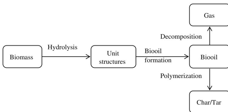
**Fig. 8.5** Conversion of cellulose to bio-oil
