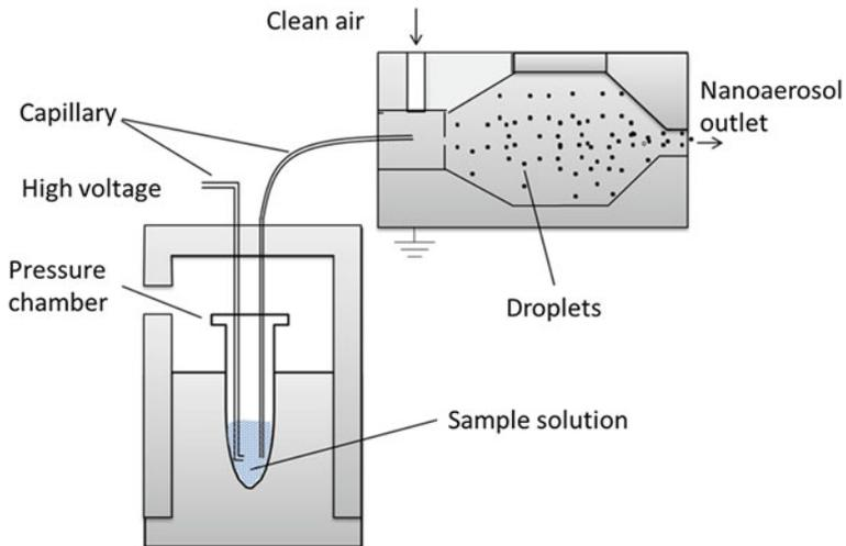
**Fig. 13.10** Electrospray technique for nanoaerosol generation [15]
