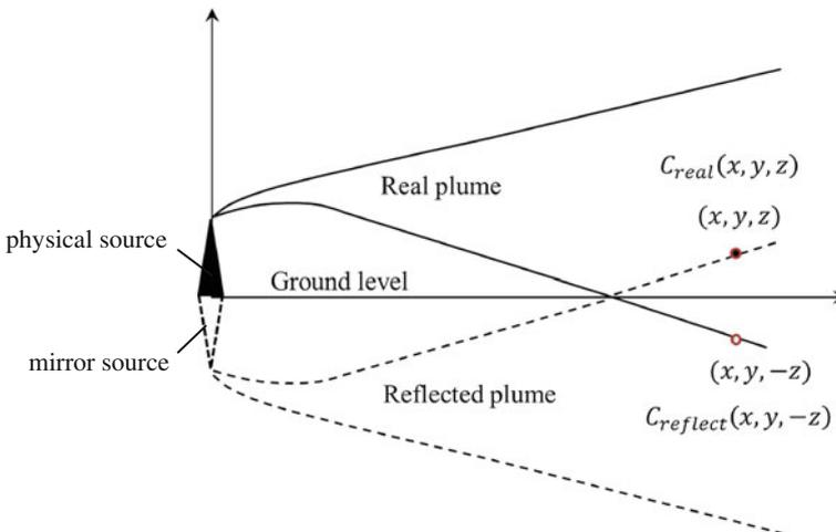
Fig. 11.12 Plume reflection on the ground surface
