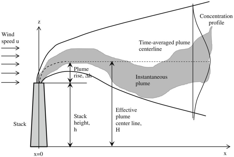
Fig. 11.7 Schematic representation of Gaussian plume dispersion
