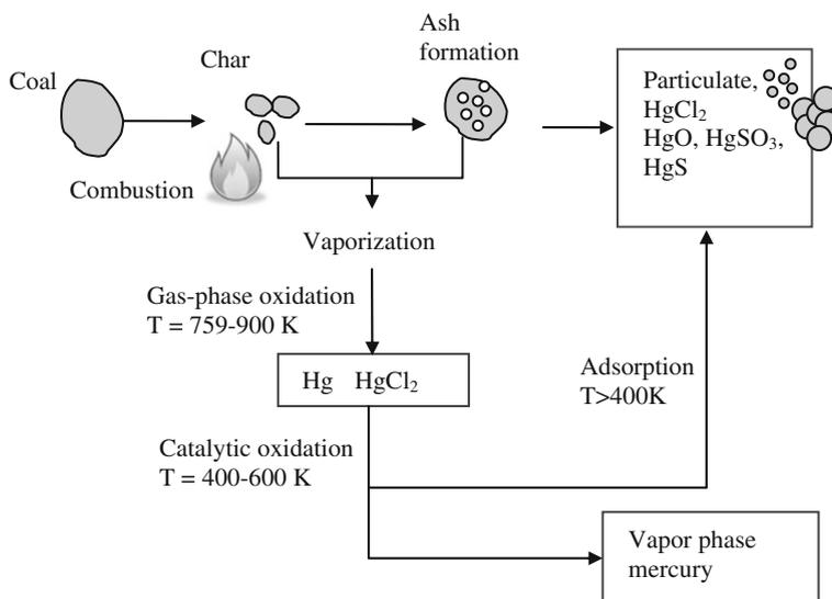
Fig. 7.8 Most probable mercury-species transformations in- and post- coal combustion
