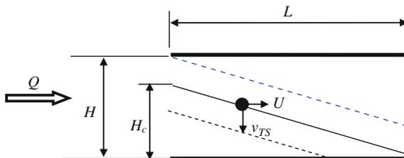
Fig. 6.2 A laminar flow gravity settling model
