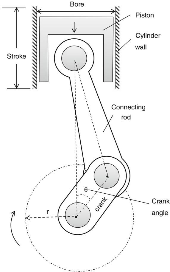
Fig. 9.2 Schematic diagram of a four-stroke piston engine
