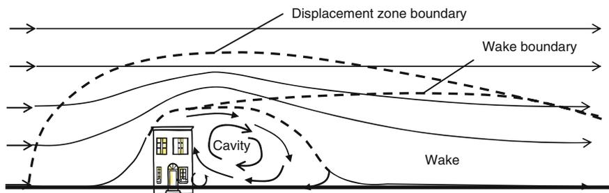
Fig. 11.11 Schematic representation of building downwash
