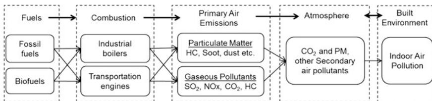
**Fig. 1.3** Fate of combustion-related air emission control
