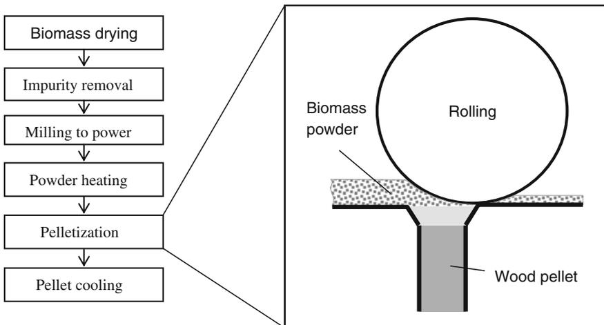
**Fig. 8.3** Pellet processing
