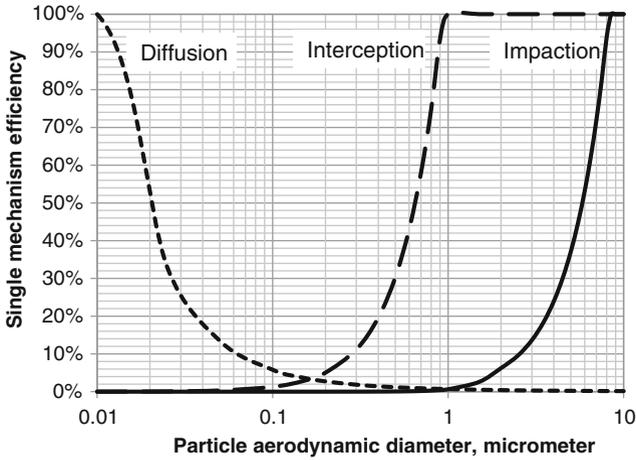
Fig. 6.12 Relative importance of different filtration mechanisms
