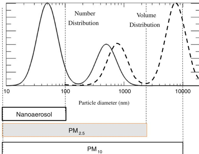
Fig. 13.2 Aerosol number and mass distribution versus size
